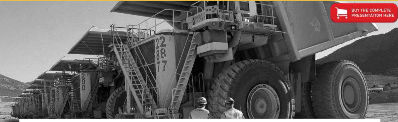
Welcome to the Hard Hat Training Series. Today, we will talk about haul trucks, also known as rock trucks. Haul trucks are heavy, earth-moving machines. To say these are big is an understatement. They can carry between 35 and 400 tons of payloads, and the cab of a haul truck is usually 3-5 meters above the ground. These goliaths are considered the workhorse of a mining operation.
